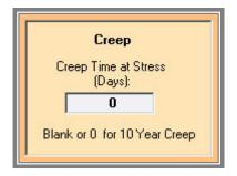
Entering a number in Creep Time at Stress (Days) lets you calculate the final creep that would result from a longer or shorter time period. A shorter time period may be helpful in evaluating conductors that have been in air for any time period less than 10 years. A longer time period may be helpful to see if any additional creep may occur if a conductor has been in the air for 20 or 30 years. Enter the time period in days. Blank or 0 will default to 10 years.
