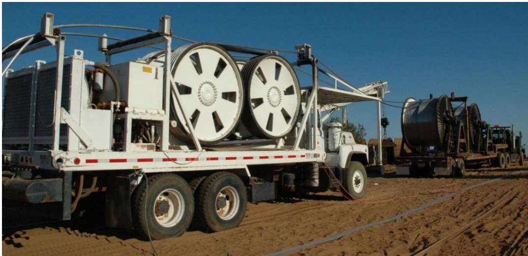
Figure 7. Dual drum bullwheel, courtesy of Oncor.
