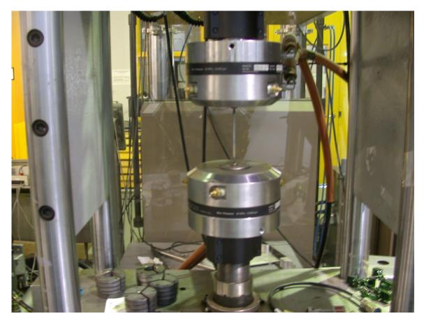
Figure 1 shows the test setup. Wire is gripped between the upper and lower grips. The upper grip is fixed while the bottom grip rotates.
