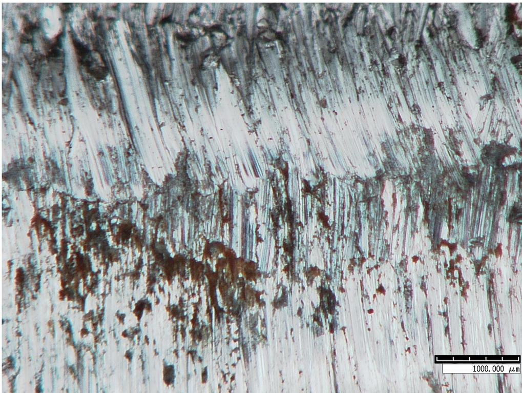
**Figure 12: Image of Scratched Special 0.1493" Wire Sample at 200X Before SCC Testing**
