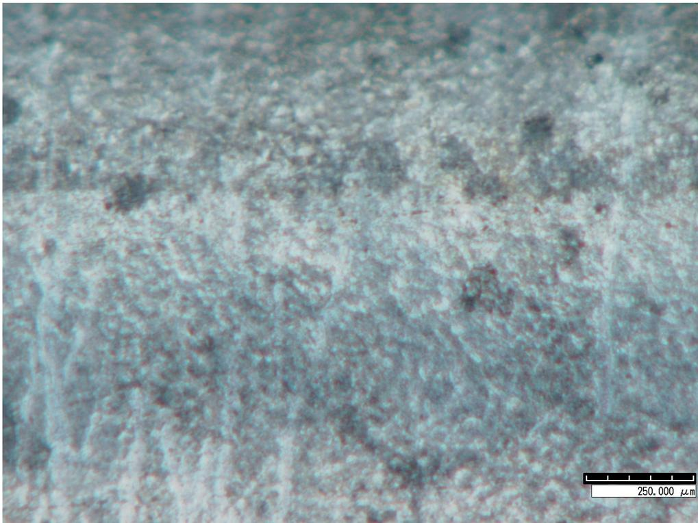
**Figure 10: Image of Special 0.1493" Wire Sample at 200X Before SCC Testing**
