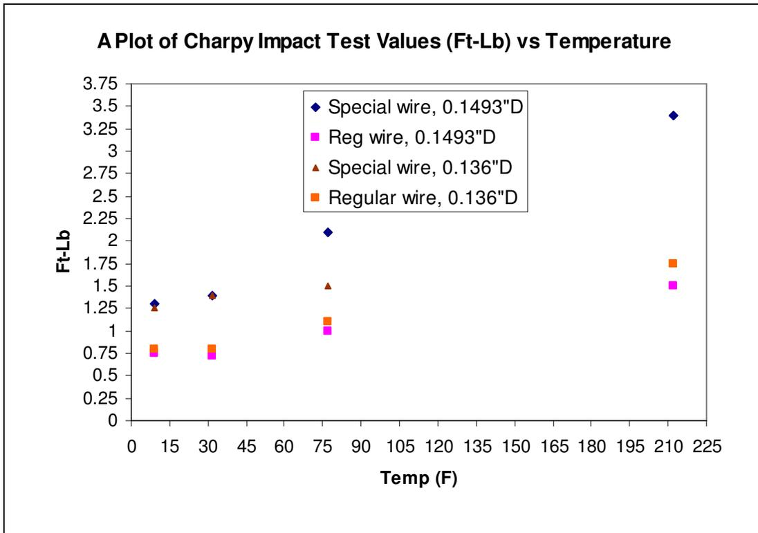
Figure 3: Charpy Impact Energy for Fracture Data for Wire Samples Versus Test Temperature
