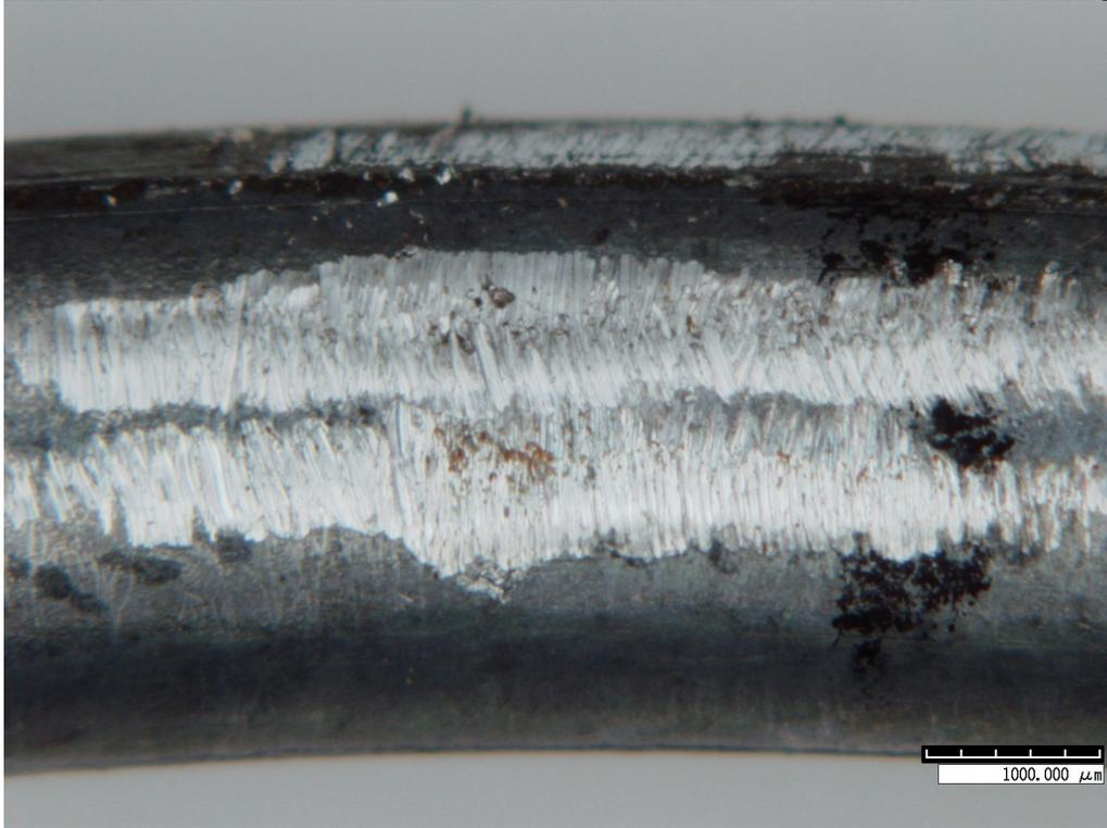
**Figure 11: Image of Scratched Special 0.1493" Wire Sample at 50X Before SCC Testing**
