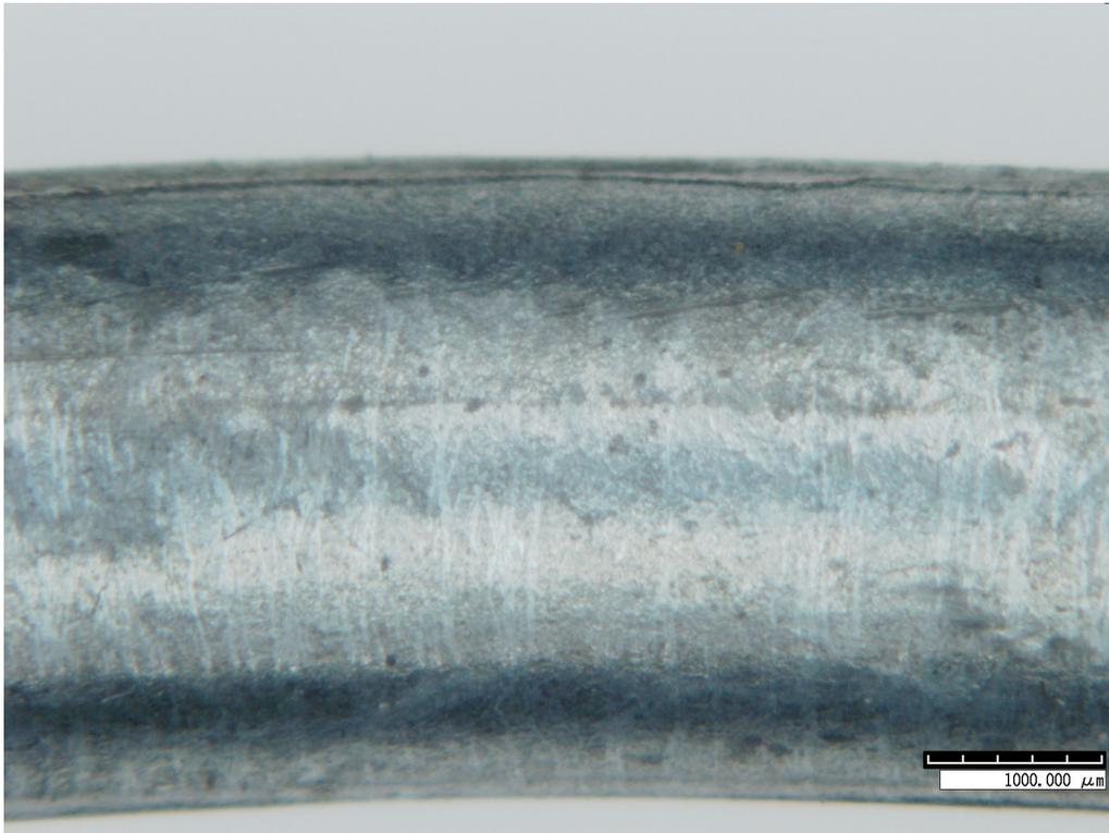
**Figure 9: Image of Special 0.1493" Wire Sample at 50X Before SCC Testing**
